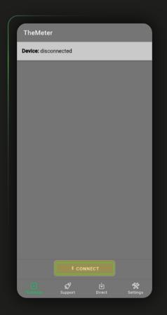
To connect your smartphone turn on the **CUBE** pro holding down the button A  $\bigcirc$  until the led turn green, then click **\*** connect on the application
