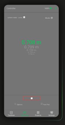
3. Rangefinder 🐼 and Real-Time 🔃 acquire any distance in single or continuous mode
